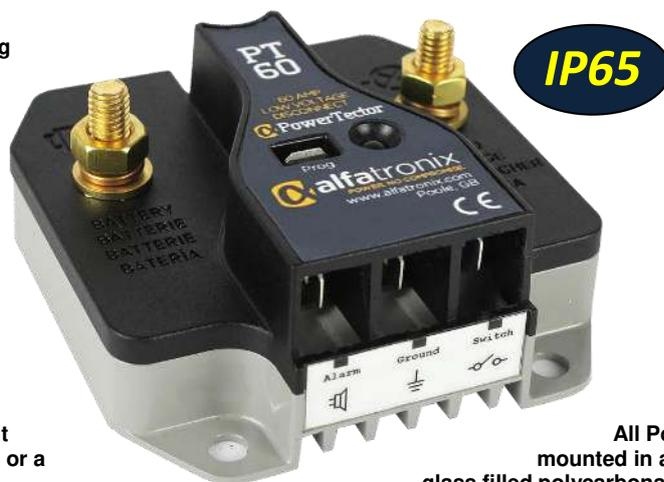
All PowerTectors from 40A upwards are mounted in a rugged die cast aluminium casing with glass filled polycarbonate cover providing terminal protection and insulation. Smaller units; 10A and 20A, are available in a lightweight, polycarbonate casing that can be simply fitted in line, like an inline fuse without the need to drill the vehicle chassis.
